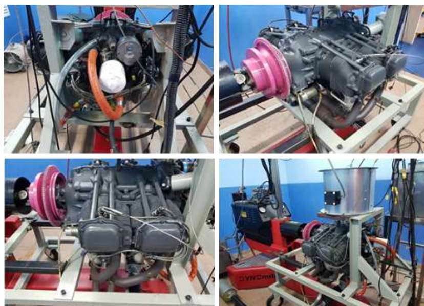
Figure 2: Engine set-up with Dynamometer
