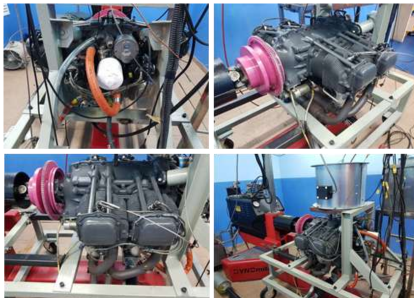
Figure 2: Engine set-up with Dynamometer
