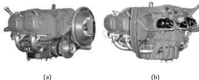
Figure 1: Typical O-320 Series (a) \frac{3}{4} Right Front View (b) \frac{3}{4} Left Front View
